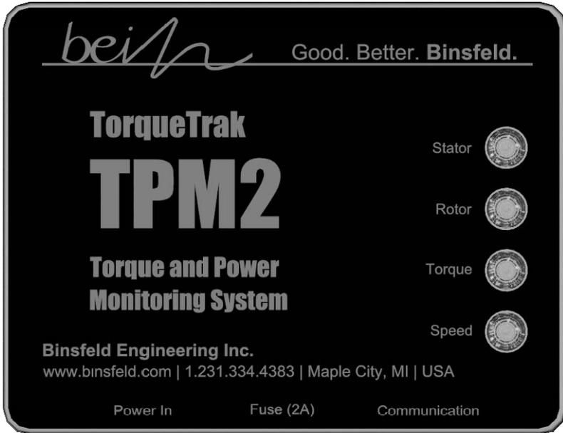
Figure 4 - Stationary Interface Faceplate
